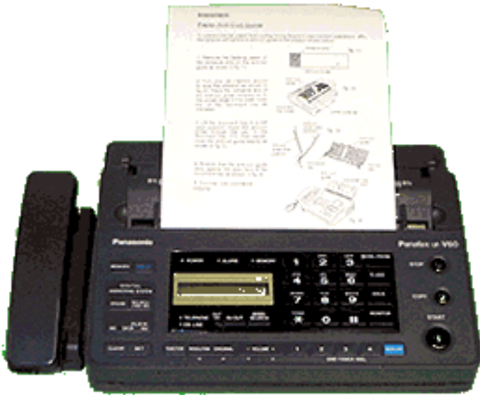
A Fax Machine uses a Thermal Printer
