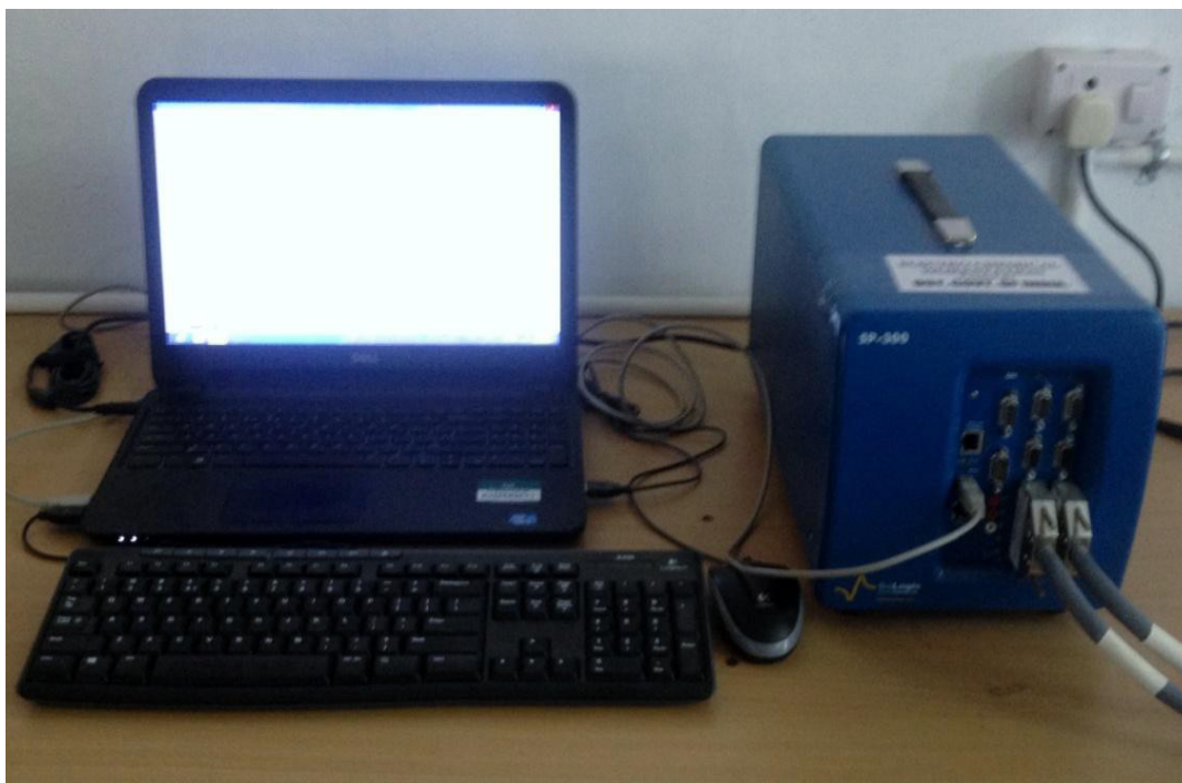
Figure 3.13. Bio logic sp-300 electrochemical work station
