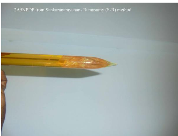
Fig. 5.5 As grown 2-amino-5-nitropyridinium dihydrogen phosphate (2A5NPDP)NLO single crystal from Sankaranarayanan-Ramasamy (SR) method
