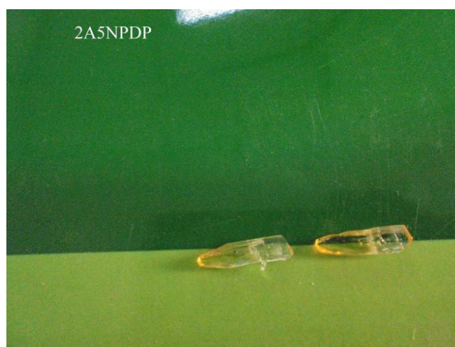
Fig.5.2 As grown 2-amino-5-nitropyridinium dihydrogen phosphate (2A5NPDP)NLO single crystal from slow evaporation method.
