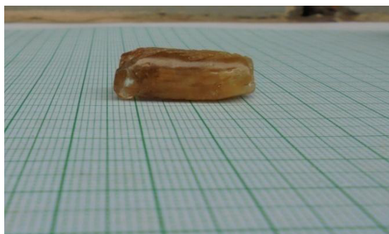
Fig. 4.4 (b) As grown NLO single crystal of 2-amino -5-nitropyridinium chloride (2A5NPCl) from assembled temperature reduction (ATR) method
