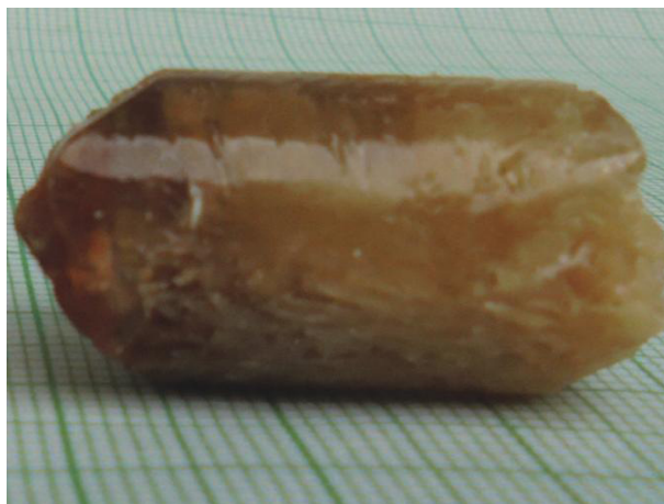
Fig. 4.4 (a) As grown NLO single crystal of 2-amino -5-nitropyridinium chloride (2A5NPCl) from assembled temperature reduction (ATR) method
